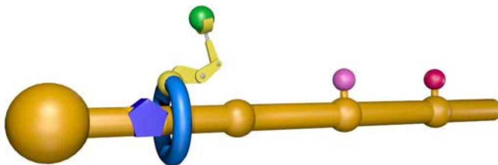
With molecules for moving parts, this nanorobot links together amino acids (colored balls) by attaching them to a moving ring (blue). Credit: Miriam Wilson
